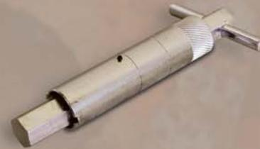
**Fig. 9 - Tool to Raise or Lower Spout Height on B2305 and B2311**
