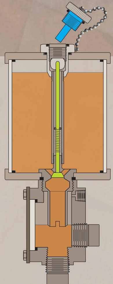
**Fig. 12 - Oil Retention During Reservoir Refills**
