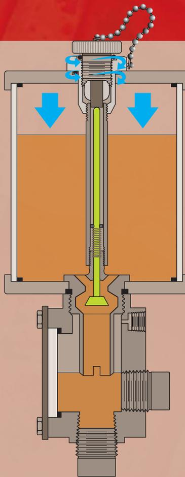
A partially open cap allows air (blue) to flow past the threads
