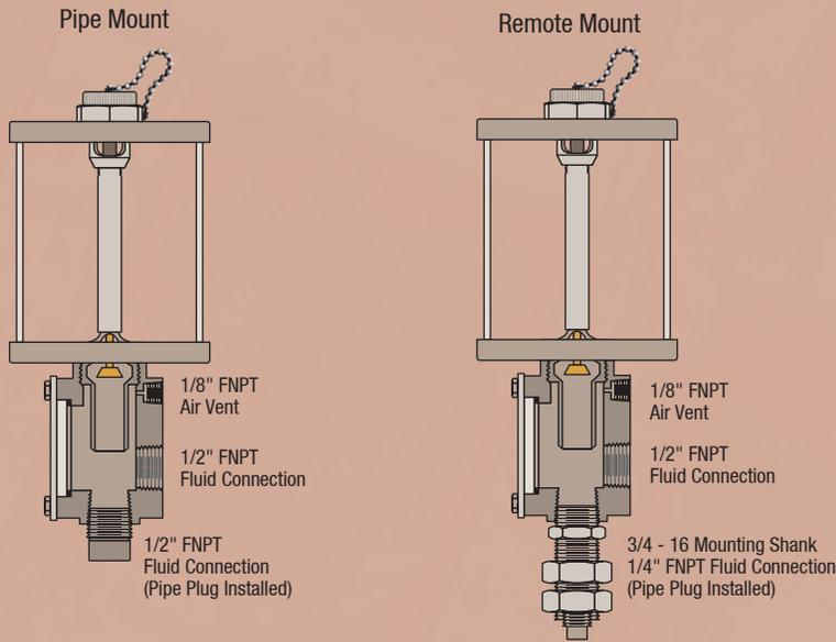
**Fig. 7 - Style C Connections and Mounting Options**
