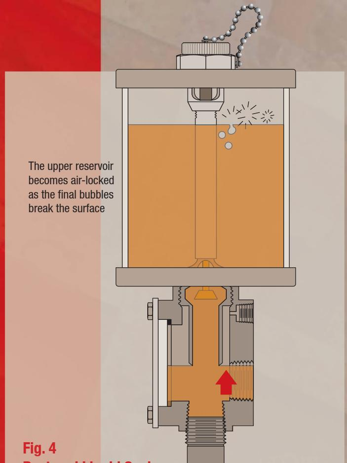
The upper reservoir becomes air-locked as the final bubbles break the surface
