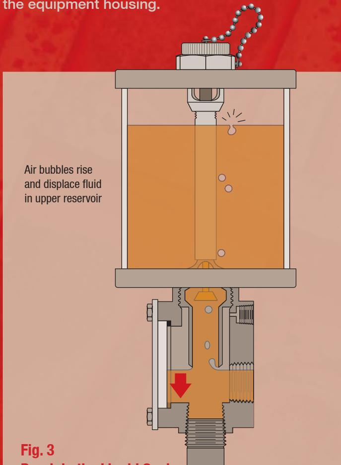
Air bubbles rise and displace fluid in upper reservoir
