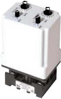
Dual adjustments along with dip switches permit accurate settings for most applications. A chart for switch positioning is printed on timer for ease in selecting time ranges. 120 Volts, 60 Hz standard.
