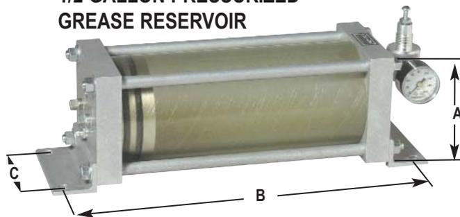
This reservoir uses pressurized air, acting on a piston, to pressurize the grease. The unit is supplied with a built in air regulator and pressure gauge for easy adjustment. The reservoir is designed for 100 PSIG operating pressure. A safety relief valve, on the grease side, is set at 120 PSIG to prevent over-pressurization. Filling the unit through the built in grease fitting is quick and easy. The unit has (3) 1/4" NPT outlets.
