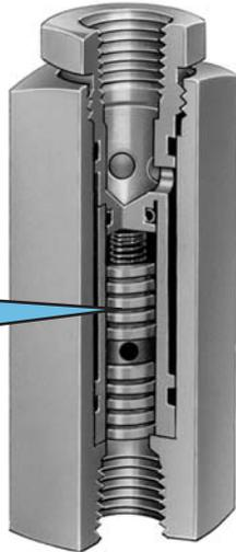
Piston increases or decreases the area of the outlet port of the cylinder, furnishing a constant flow rate under varying pressure.
